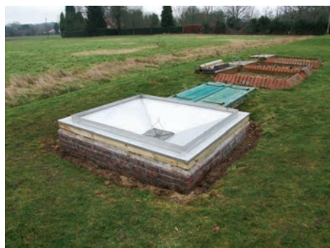
Figure 2. (a) The one thousandth of an acre rain gauge with drain gauges behind
