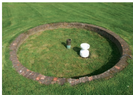
Figure 2. (b) Turf wall enclosure with five inch cylindrical rain gauge (centre) and new aerodynamic ARG100 tipping bucket rain gauge
