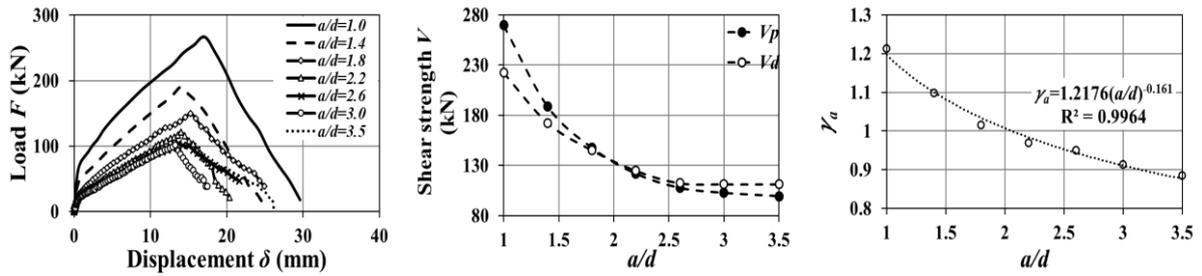
(a) Mean of the 30 samples with different  $a/d$  (b) Variation in shear strength with  $a/d$  (c) Variation in  $\gamma_a$  with  $a/d$
