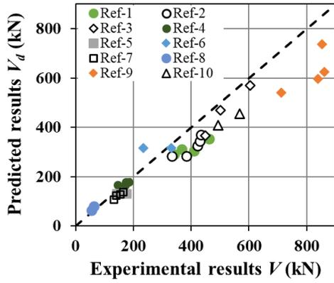
(a)  $V_d$  calculated by Eq. 6 compared with experimental results
