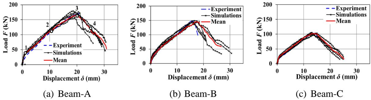
652 **Figure 11.** Simulated shear load-displacement curves in comparison with experimental
