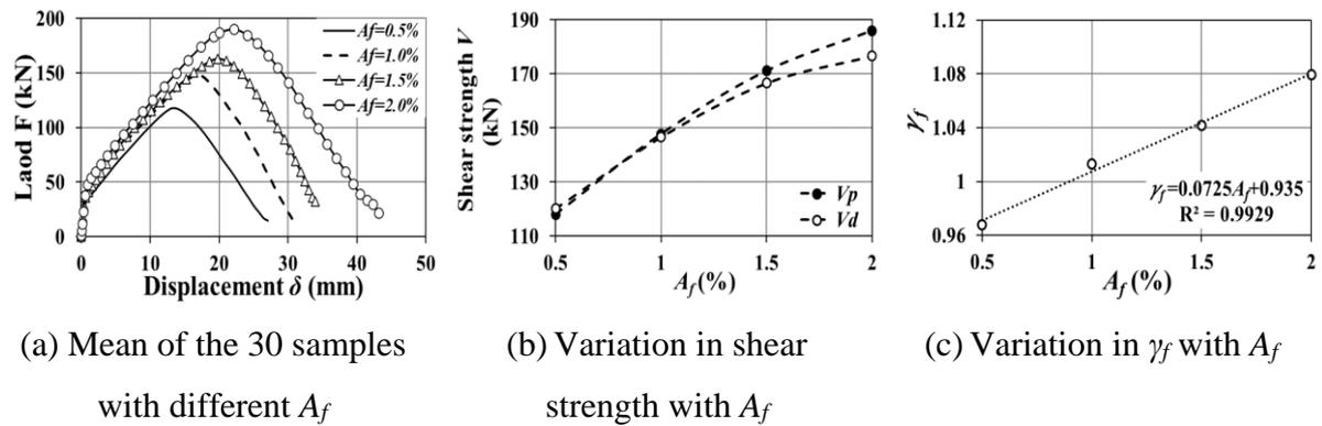
660 **Figure 16.** Change in load with displacement for different  $A_f$  (a); changes in the shear
