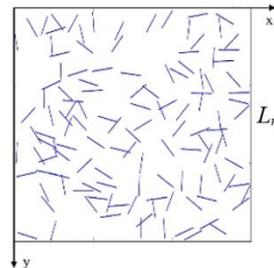
(d) The projected  $N$  fibres is modified to  $N_{2D}$  fibres based on their length  $L_f$  used in 2D models
