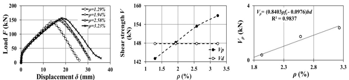
(a) Mean of the 30 samples with different  $\rho$  (b) Change in shear strength with  $\rho$  (c) Change in  $V_\rho$  with  $\rho$
