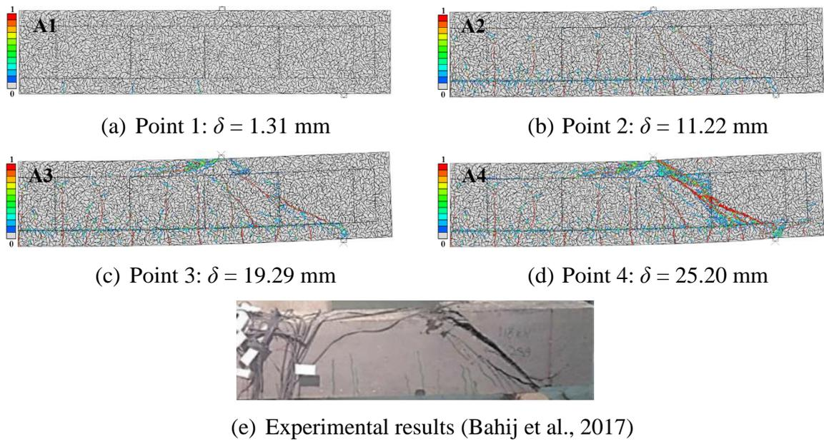
654 **Figure 12.** Simulated cracking process and pattern in comparison with experimental data for
