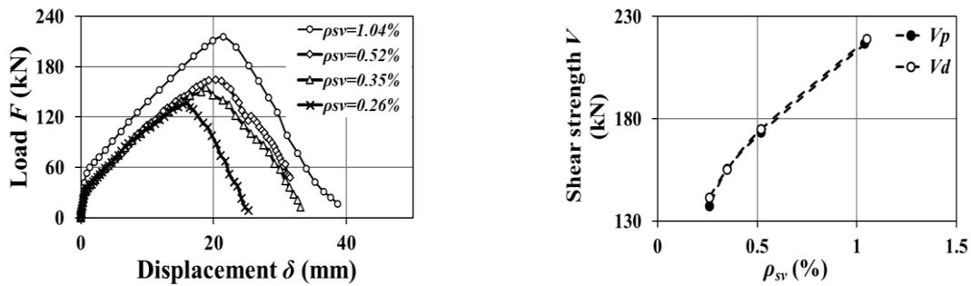
(a) Mean of the 30 samples for different  $\rho_{sv}$  (b) Change in shear strength with  $\rho_{sv}$
