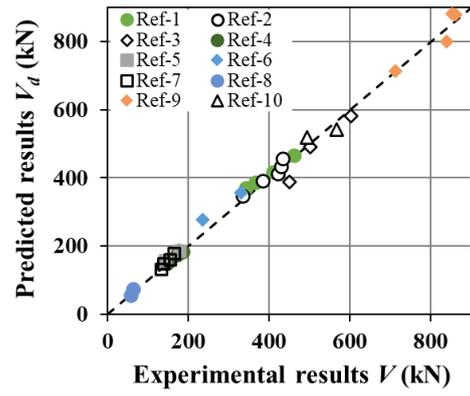
(b)  $V_d$  calculated by Eq. 14 compared with experimental results
