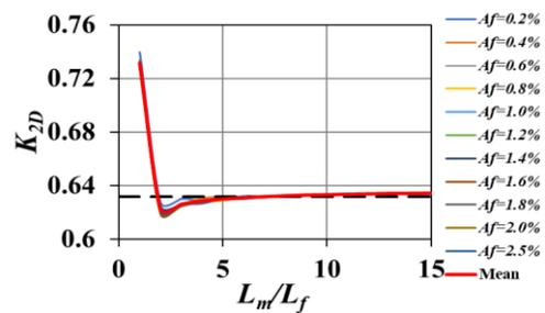
(b) Mean  $K_{2D}$  of the 9000 samples with different  $A_f$
