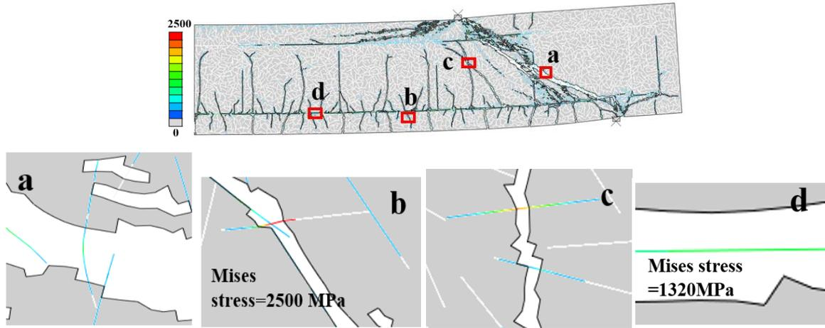
658 **Figure 14.** Cut-off views of simulated failure modes (Figure 12d) for Beam-A in Example 2.
