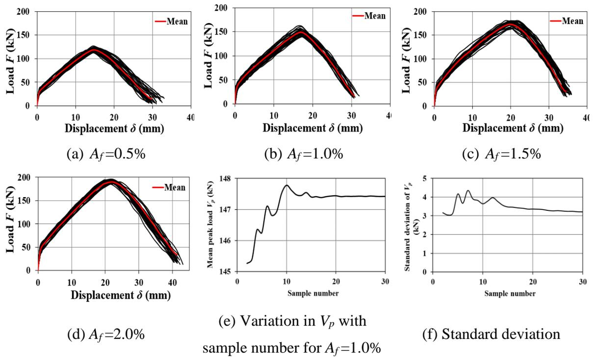
659 **Figure 15.** The shear load-displacement curve simulated for the 30 samples with different  $A_f$
