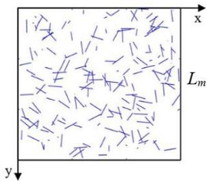
(c) The projected  $N$  fibres in the 2D plane
