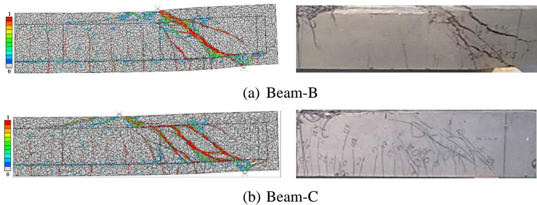
656 **Figure 13.** Simulated final crack patterns in comparison with experimental data for Beam-B
