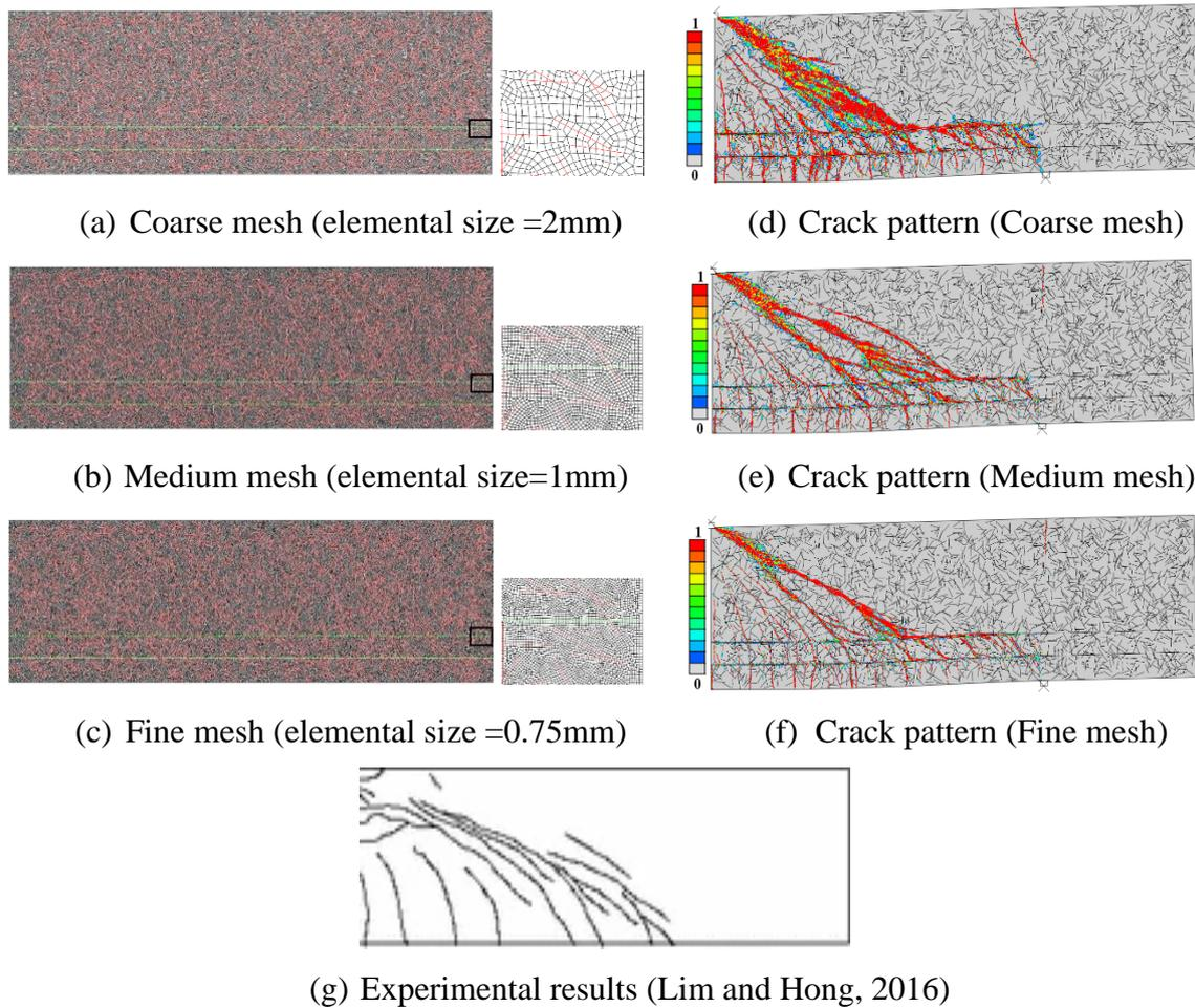
643 **Figure 6.** The three FE meshes (a-c), and the simulated final crack patterns (d-f) for Example
